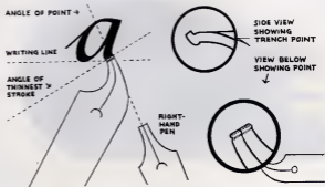
Fig. 8: Designed by Piggott, built by Osmiroid: the nib with a hook for "hooked" lefties.
